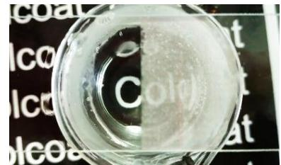
Curing Condition : 125 °C, 1 min (bar coater #5)
